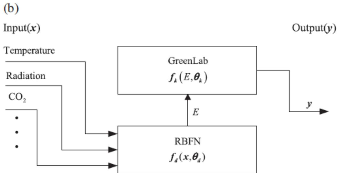
Fig. 2. The knowledge-and-data-driven model (KDDM) with two cases of coupling: (a) superposition coupling operator and (b) composition coupling operator.
